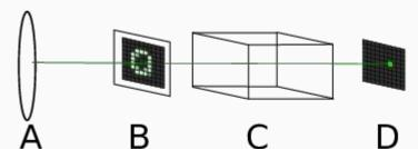
Laser illuminates screen, photon travels to single-photon detector array (SPAD), provably-optimal accuracy is MLE, *hard upper bound of 22.96%* for MNIST, "with cheating" i.e. achieved when training on the test set.
