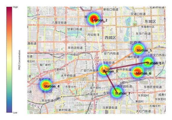
The figure shows the predicted PM25 concentrations of the AirPhyNet model at particular timestep by a heatmap and the diffusion from station\_3 to its neighboring stations by different line segments. The magnitude of diffusion is reflected by the line color.
