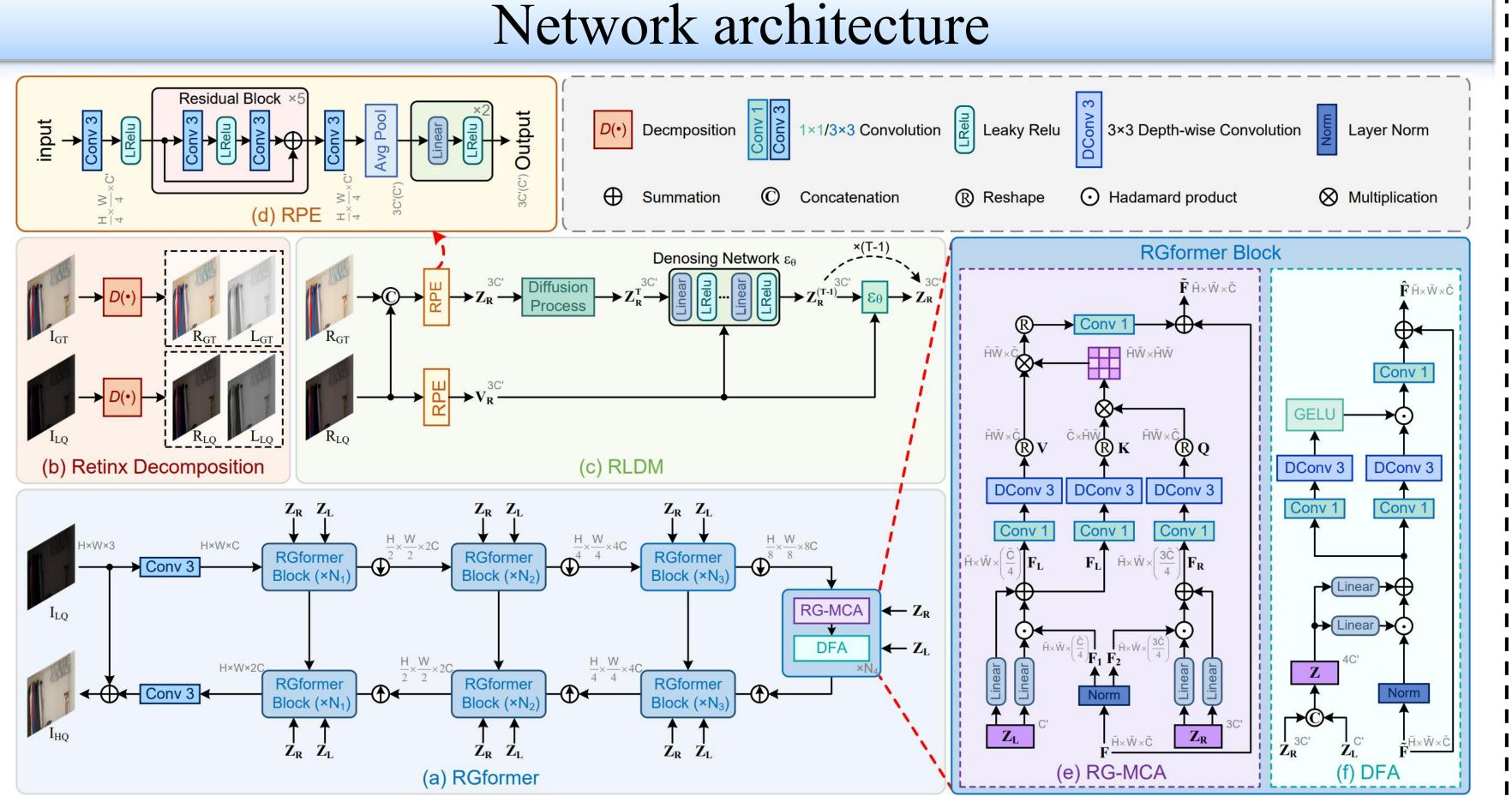
Framework of our Reti-Diff. In Phase I, we pretrain Reti-Diff with RGformer and RPE to ensure the robust learning of RLDM. In Phase II, we optimize RLDM to generate high-quality Retinex priors to guide RGformer in detail enhancement and illumination correction.
