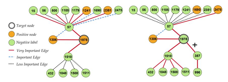
The computation graph for the targeted node 1978 from the CORA datasets, as identified by GNNExplainer. The edge (1978, 387) is added during the successful attack. Edge importances change considerably after the attack and negative class gains importance due to the newly added nodes.
