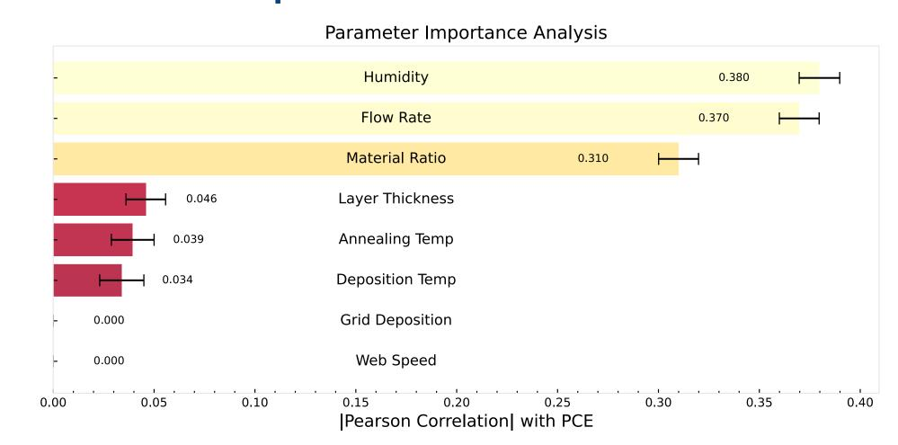
• High humidity correlation (r = 0.38) and system tolerances created a noisy, locally complex space. This made RS more effective than BO under real-world conditions.
