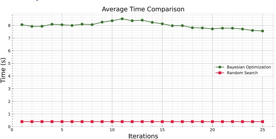
BO required ~8 seconds per iteration making it ~20× slower than RS, which averaged ~0.4 seconds per iteration.
